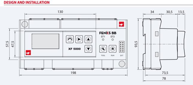
Controller can be snap-mounted on DIN rail (35 mm) or screwed directly to a mounting plate using two holes on the case.
